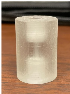
Figure 7: Nozzle Hub. The hub has two \frac{1}{4} "-28 threaded holes with a 1.5875 mm channel. Provides a modular bottom connection to several nozzles (i.e. Shower Head or Jet)
