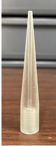
Figure 5: Aspiration Nozzle, meant to aspirate the well volume after applying mixing recipe.
