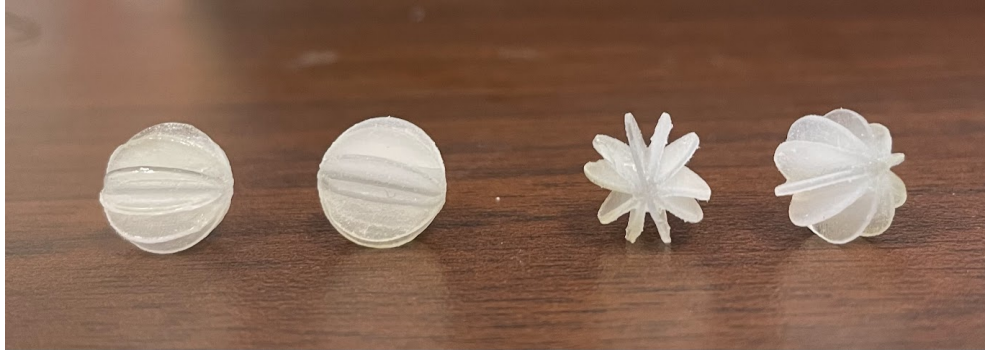
Figure 22 : Propeller Balls manufactured through polyjet printer ( Material : VeroClear )
